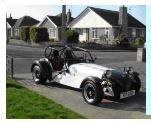
My Superlight Caterham 7 R500 Weighing 460 Kilos with power @ 255 BHP @ 8600 RPM = 562 BHP per Tonne and 0-60 MPH 3.2 seconds
